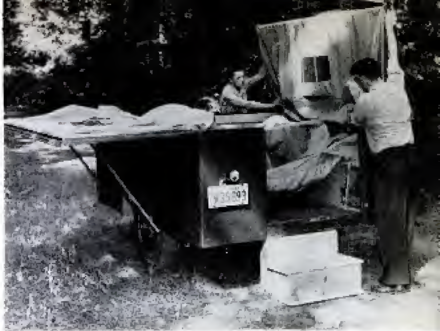
To set up camp, wings of trailer to which tent is attached are first opened outward and supported by fold-away pipe braces
